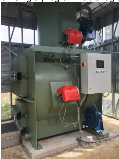
Typical CA Model Incinerator. Showing Loading and ash Removal doors. Primary and Secondary Burners, Combustion Air fans and Control Panel.
