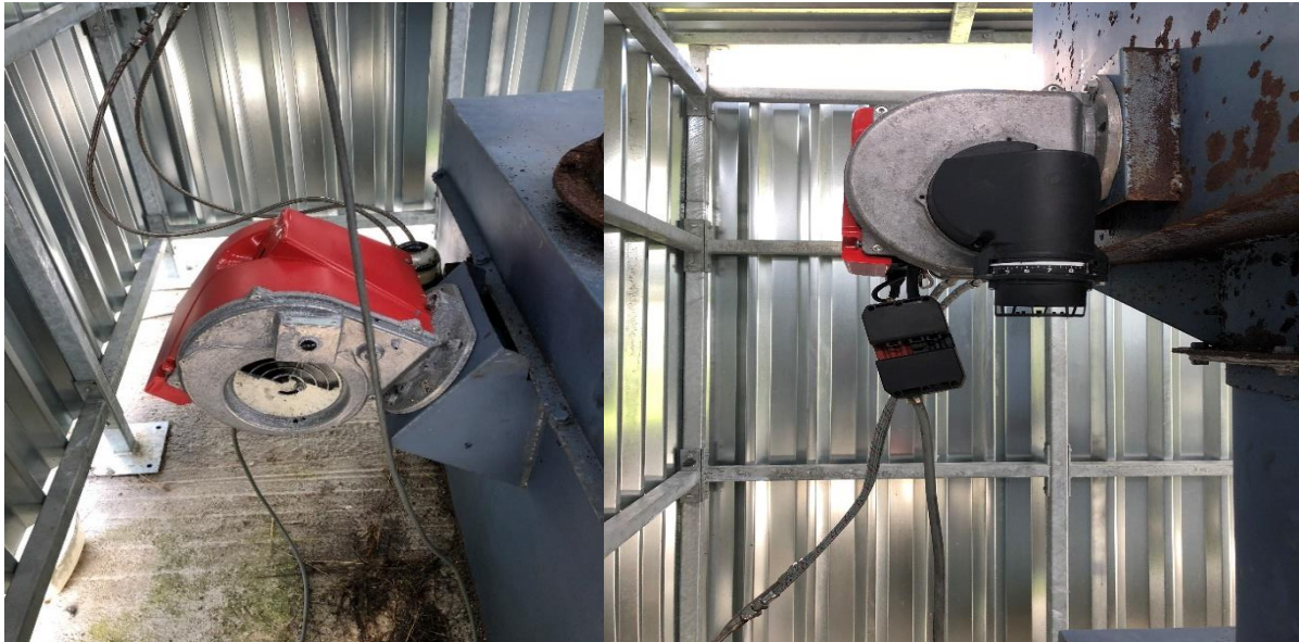
Inciner8 i8-75a primary and secondary burners.
